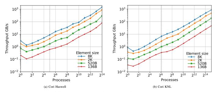
Fig. 4: Weak scaling of distributed hash table insertion. The dotted line represents the processes in one node.
