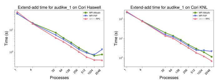
Fig. 8: Strong scaling of extend-add on Cori Haswell (left) and Cori KNL (right).
